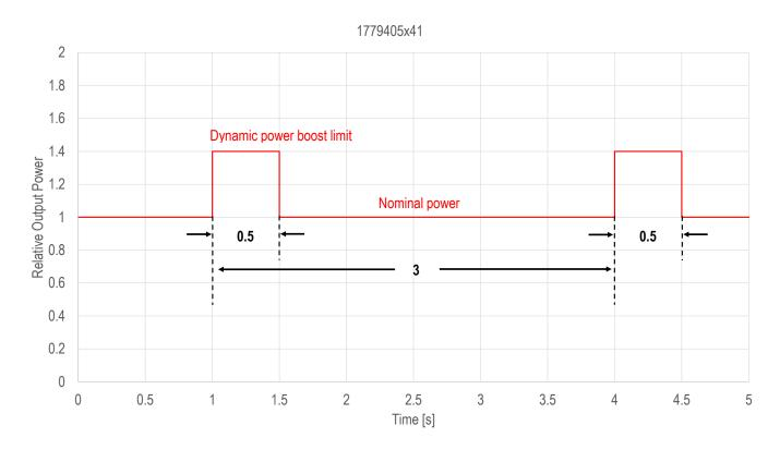
**Note:** The overload current of 140% of  $I_{OUT}$  can be supplied for maximum 0.5s and requires a 3s recovery time till next overload event.
