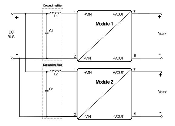
As a starting point for the decoupling filters, use the values of the reference filters - see also "RADIATED AND CONDUCTED EMISSIONS (WITH EMI INPUT FILTER)". The final appropriate filter for the application has then to be evaluated under operation in the target application by checking e.g. the change of the input ripple voltage.
