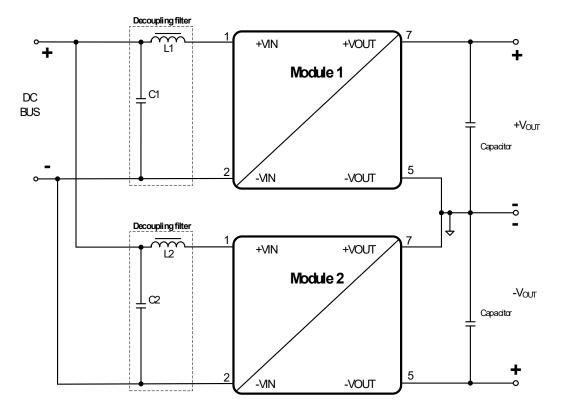
For using long supply lines or different line length for each 1779405x41 it is recommended to decouple each power module with an additional LC- filter. The decoupling LC-filter is also recommended if the supplying dc bus has a high impedance so that high voltage swings at the input of each power module could be present. As initial values, the EMI filter shown for every part number can be used. See also "Primary side parallel connection".
