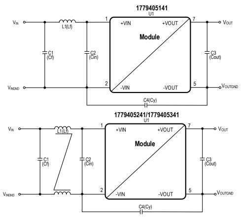
For optimal EMI performance, one filter capacitor, C1, one filter inductor / common mode chocke (cmc), L1, one input capacitor, C2, one output capacitor, C3 and one Y-Cap, C4 are recommended. For optimal electrical performance, one input capacitor C2 and one output capacitor C3 are recommended.
