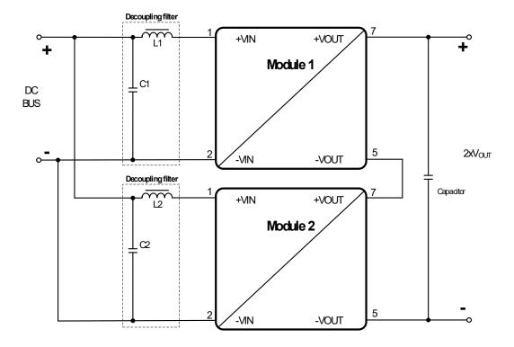
In case of using long supply lines or different line length for each 1779405x41 it is recommended to decouple each power module with an additional LC filter. The decoupling LC filter is also recommended if the supplying dc bus has a high impedance so that high voltage swings at the input of each power module could be present. As initial values, the EMI filter shown for every part number can be used. See also "Primary side parallel connection".
