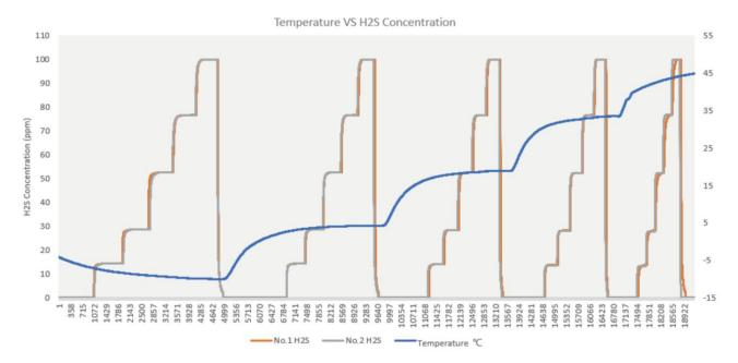
(Temperature:-15,-5,5,15,25,35,45,55°C, Gas chamber space 0.03m<sup>2</sup>, ventilation system ventilation flow 3000sccm)
