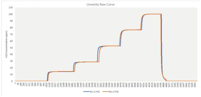
(Temperature:25 °C, Hmidity:55%, Gas chamber space: 0.03m<sup>2</sup>, Ventilation system with ventilation flow 4000sccm)
