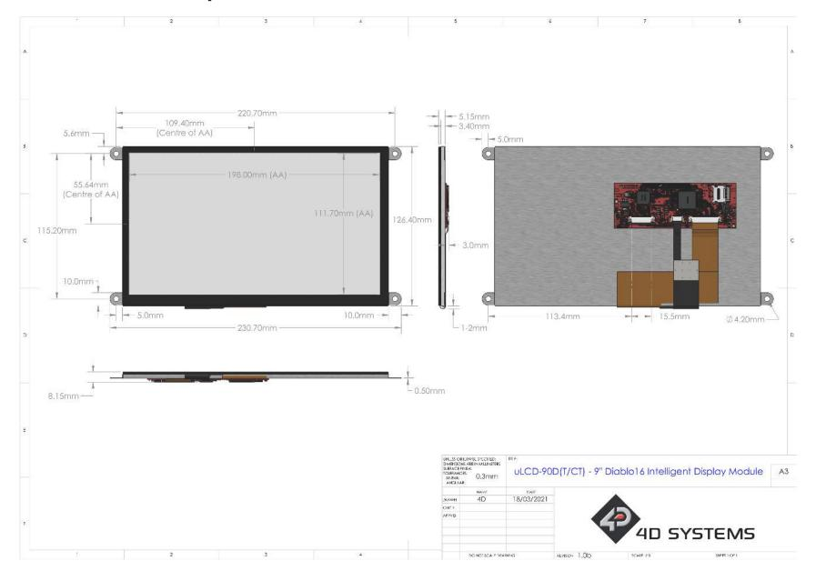
uLCD-90D Series Schematic Details (HW REV 1.5)
