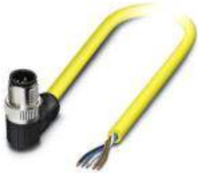
Sensor/Actuator cable, 5-position, TPE, yellow RAL 1021, Plug angled M12 SPEEDCON, A-coded, on free cable end, Cable length: 5 m
