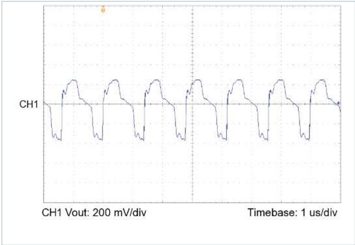
Figure 19 — Output voltage ripple, V_{IN} = 48\text{ V} , V_{OUT} = 15.0\text{ V} , C_{OUT\_EXT} = 1000\text{ }\mu\text{F} , R_{LOAD} = 0.701\text{ }\Omega
