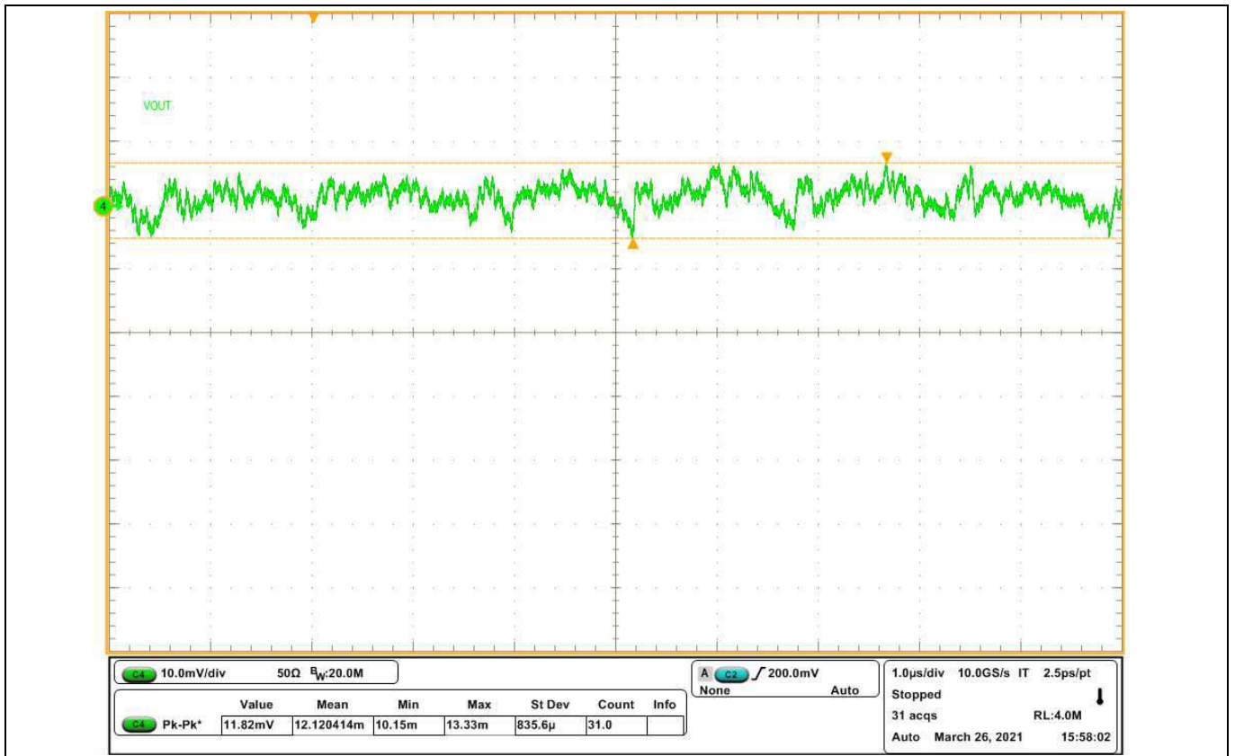
Figure 17 Vout ripple at 40 A Load, fsw = 600 kHz, (Ch4: Vo)
