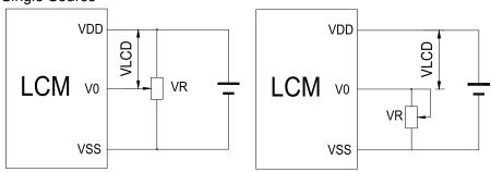
$V_{DD^{\sim}}V_0$ : LCD Driving voltage
