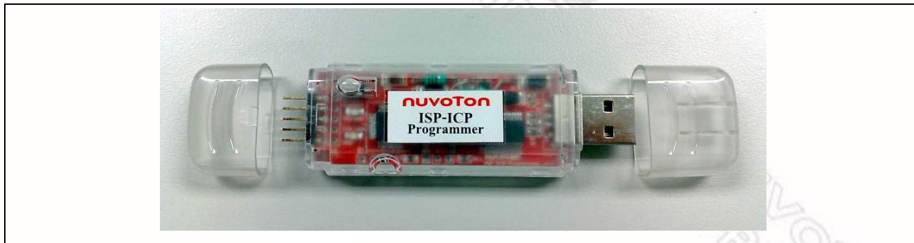
Figure 27–2 Nuvoton ISP-ICP Programmer
