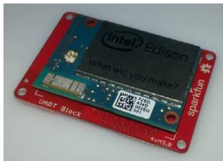
UART Block Installed
