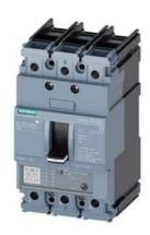
circuit breaker 3VA5 UL frame 125 3-pole, starter protection TM120M, AM, In=70A without overload protection short-circuit protection Ii=3...7 x In cable connection on both sides
