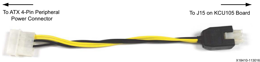
Figure E-1: ATX Power Supply Adapter Cable
