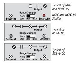
Note: Terminals are #6 screws. DC contacts are polarity sensitive.
