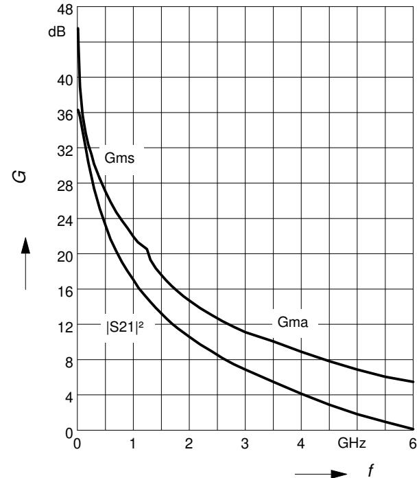
**Power gain  $G_{ma}, G_{ms} = f(V_{CE})$**
