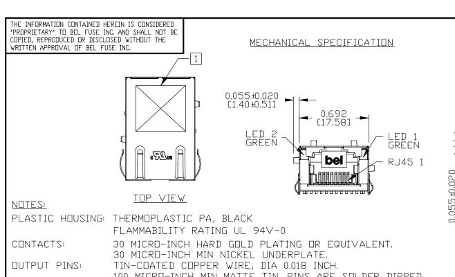
100 MICRO-INCH MIN MATTE TIN, PINS ARE SOLDER DIPPED.
