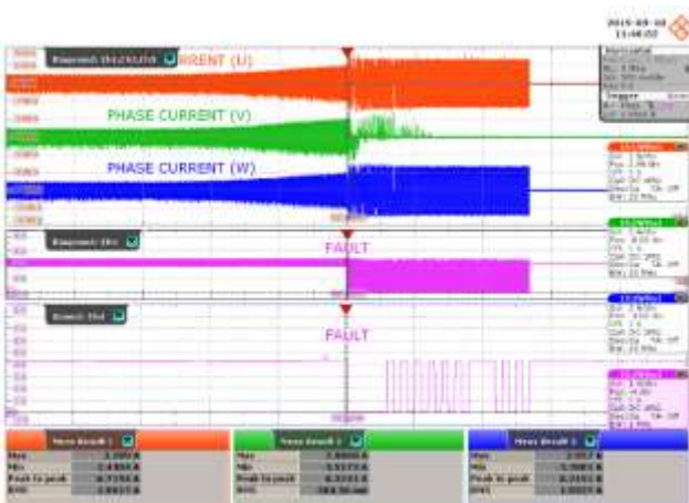
Figure 62 – At Stalled Condition, 200 W Load.
