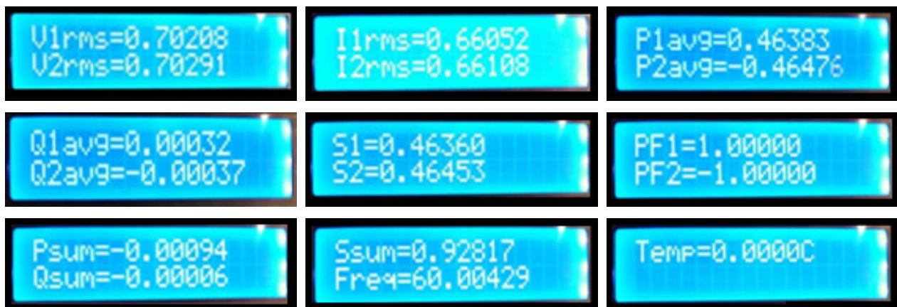
Figure 9. Standalone Power Meter Measurements
