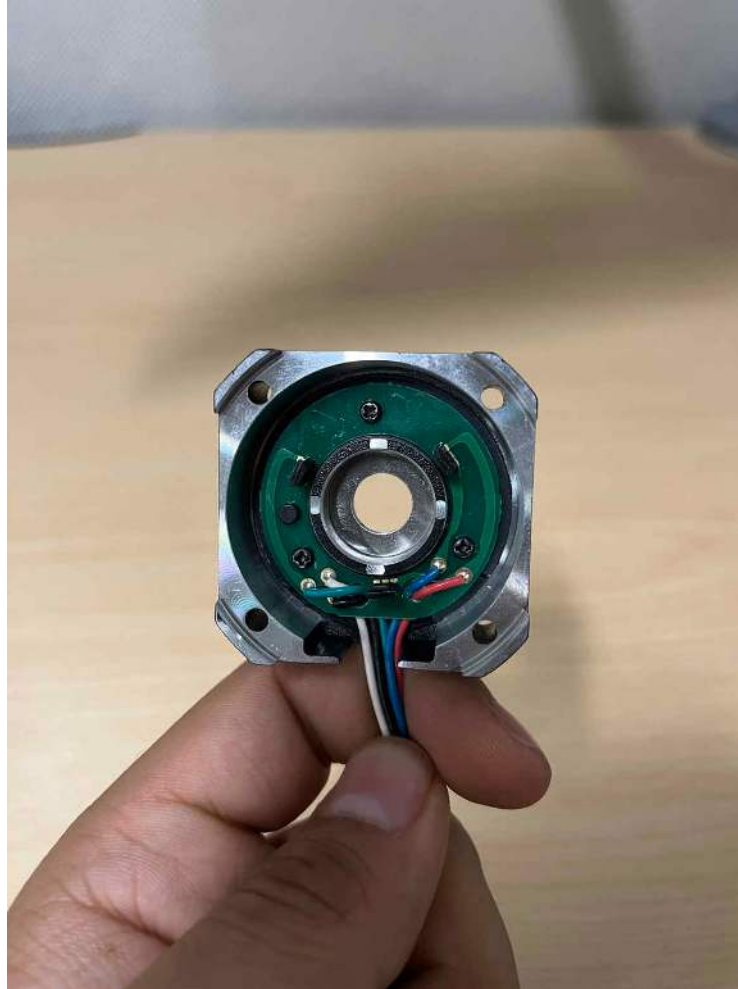
Figure 3-5. Hall Sensor Board Removal
