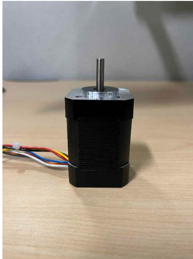
Figure 3-2. NEMA17 42-mm BLDC Motor
