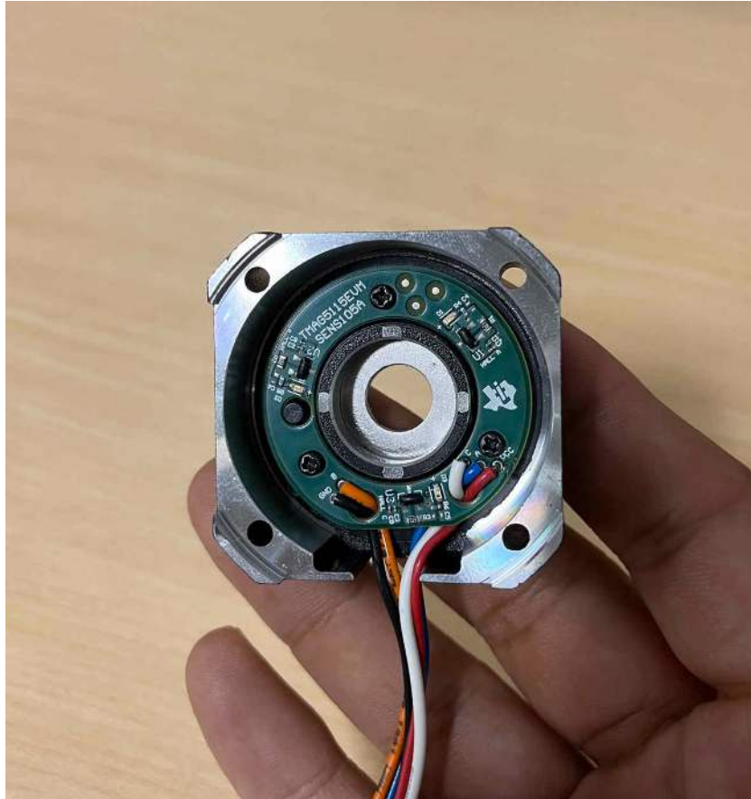
Figure 3-6. TMAG5115EVM on NEMA17 Motor Module
