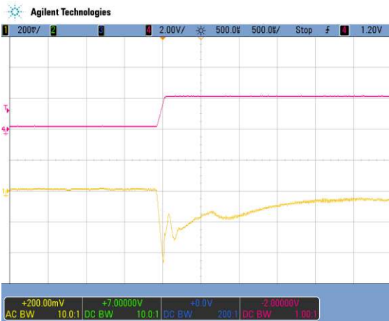
Figure 15 - Load transient V1, 3 to 125 A (500 µs/div) CH1: V1 (200 mV/div); CH4: I1 (100 A/div)
