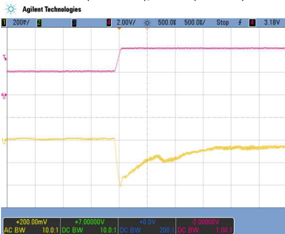
Figure 17 - Load transient V1, 122 to 244 A (500 µs/div) CH1: V1 (200 mV/div); CH4: I1 (100 A/div)
