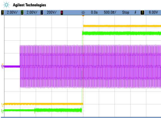
Figure 7 - Turn-On AC Line 230 VAC, full load (500 ms/div) CH1: V1 (2 V/div); CH2: VSB (2 V/div); CH3: Vin (200 V/div)
