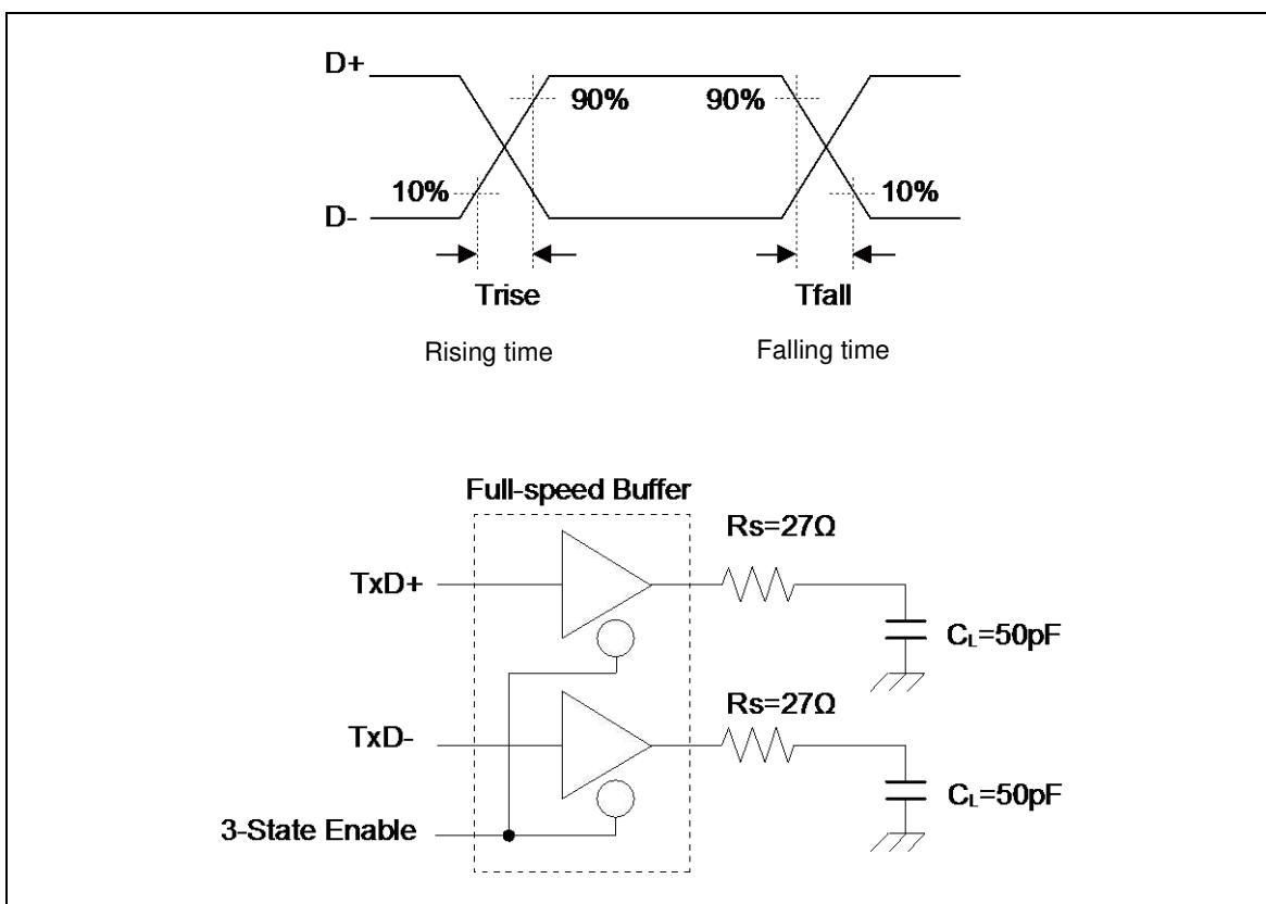
\*6: USB Full-speed connection is performed via twist pair cable shield with  $90\Omega \pm 15\%$  characteristic impedance (Differential Mode). USB standard defines that output impedance of USB driver must be in range from  $28\Omega$  to  $44\Omega$ . So, discrete series resistor ( $R_s$ ) addition is defined in order to satisfy the above definition and keep balance. When using this USB I/O, use it with  $25\Omega$  to  $30\Omega$  (recommendation value  $27\Omega$ ) series resistor  $R_s$ .
