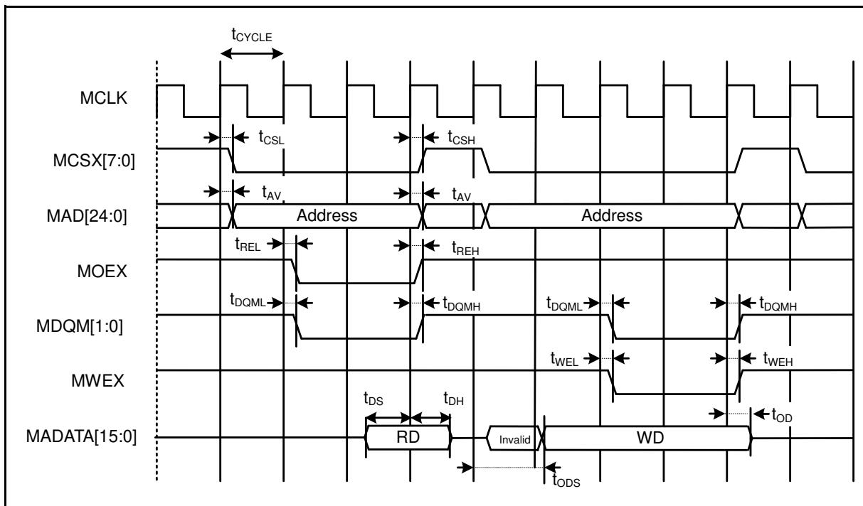
**Multiplexed Bus Access Asynchronous SRAM Mode**
