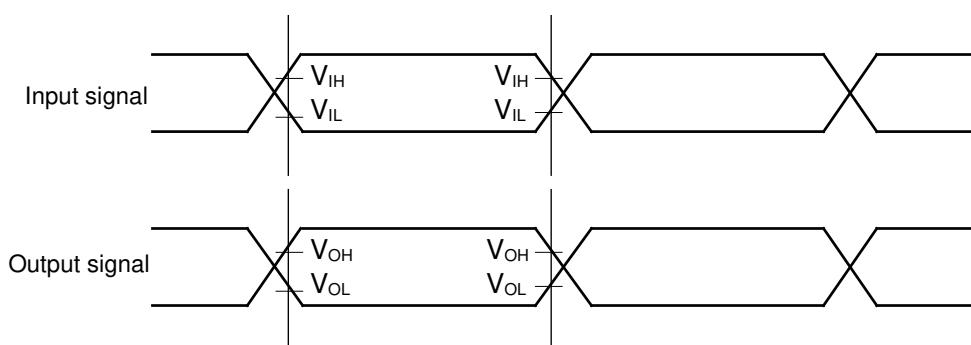
**Separate Bus Access Asynchronous SRAM Mode**
