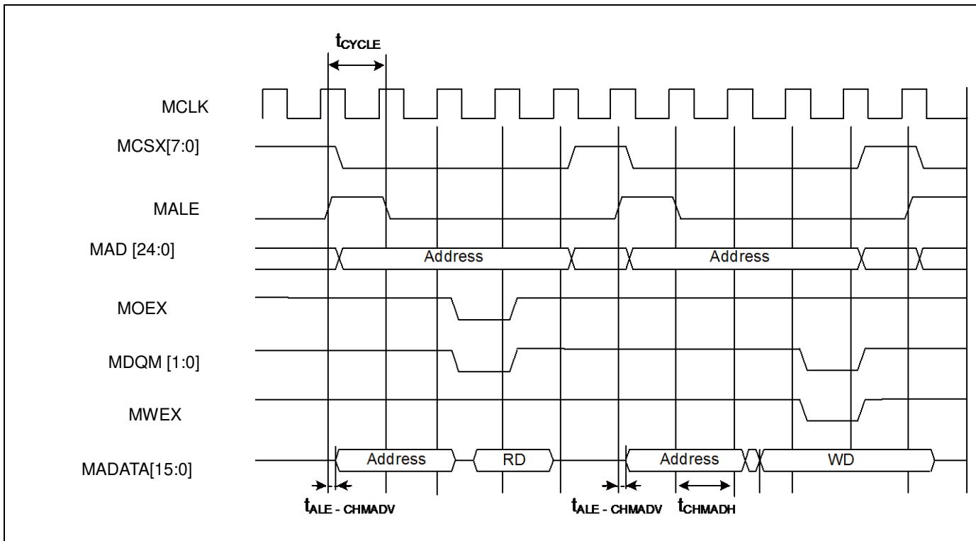
**Multiplexed Bus Access Synchronous SRAM Mode**
