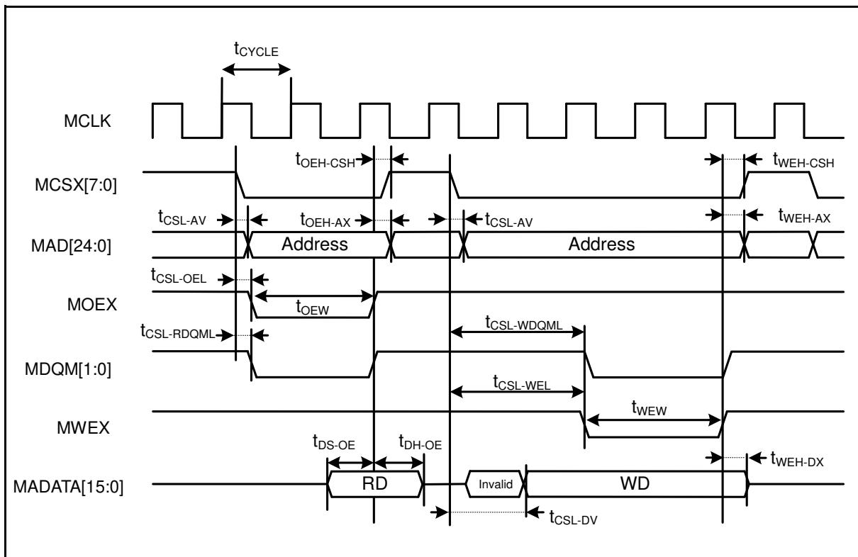
**Separate Bus Access Synchronous SRAM Mode**
