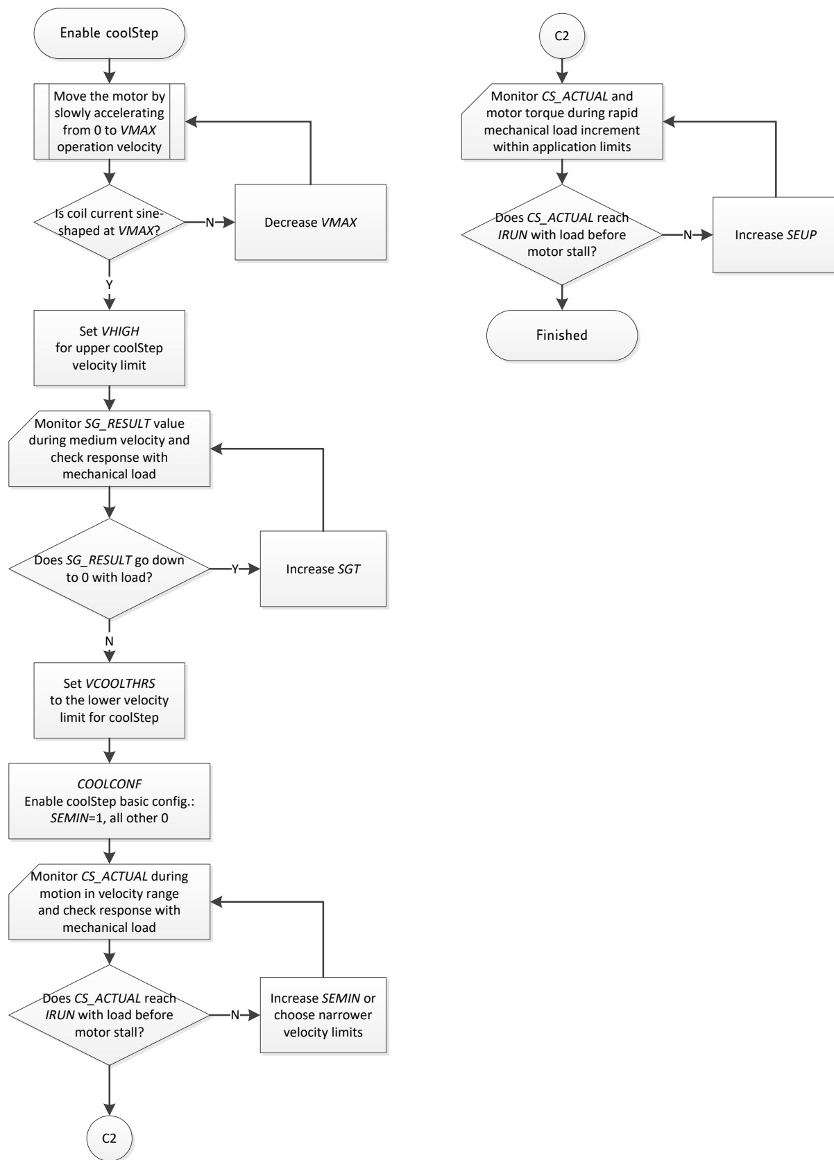
Figure 13.3 Enabling coolStep (in combination with spreadCycle)
