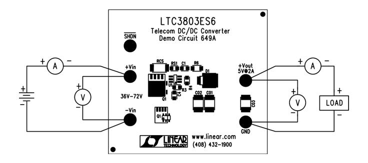
Figure 1. Proper Measurement Equipment Setup
