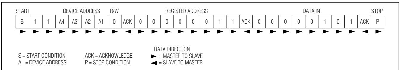
Figure 5. Example—Setting CLK3 to 80MHz
