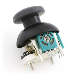
**Description:** This is a joystick very similar to the 'analog' joysticks on PS2 (PlayStation 2) controllers. Directional movements are simply two potentiometers - one for each axis. Pots are ~10k each. This joystick also has a select button that is actuated when the joystick is pressed down
