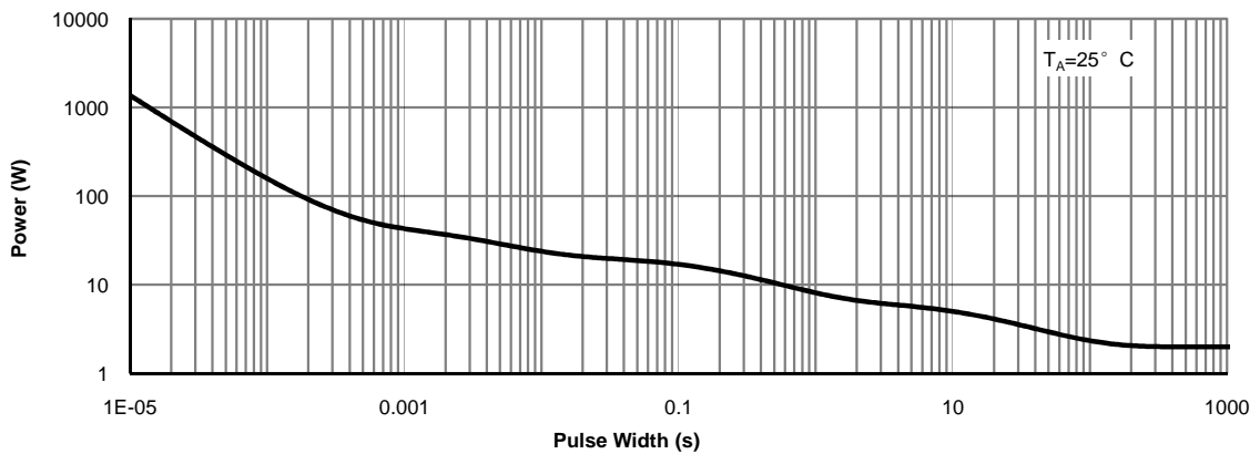
Figure 14: Single Pulse Power Rating Junction-to-Ambient (Note H)
