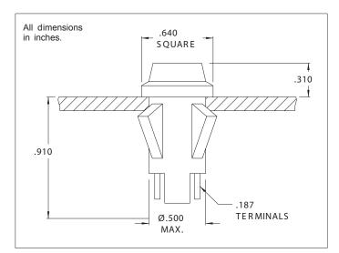
Mounting: Will snap-fit into Ø.500/.505 hole in panels .020/.100 thick. Push-on speednut SN0461 also available. Mounting hole pattern on page SP2.
