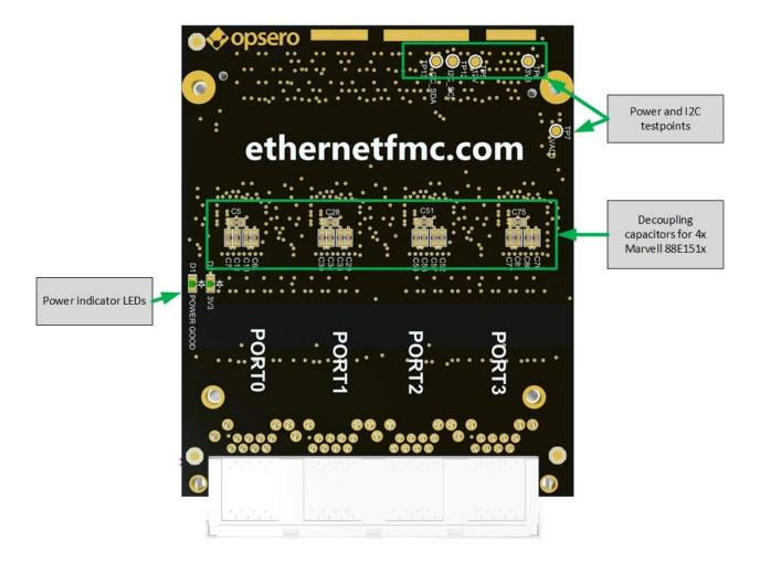
The main components on the bottom-side of the mezzanine card are:
