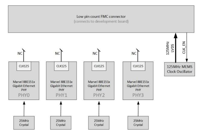
Each of the 4x 88E151x PHYs is connected to a 25MHz crystal for generation of it's own internal clocks. The Ethernet FMC also has a 125MHz MEMS clock oscillator with LVDS output to provide the FPGA fabric with a precision clock for driving the Ethernet MACs.
