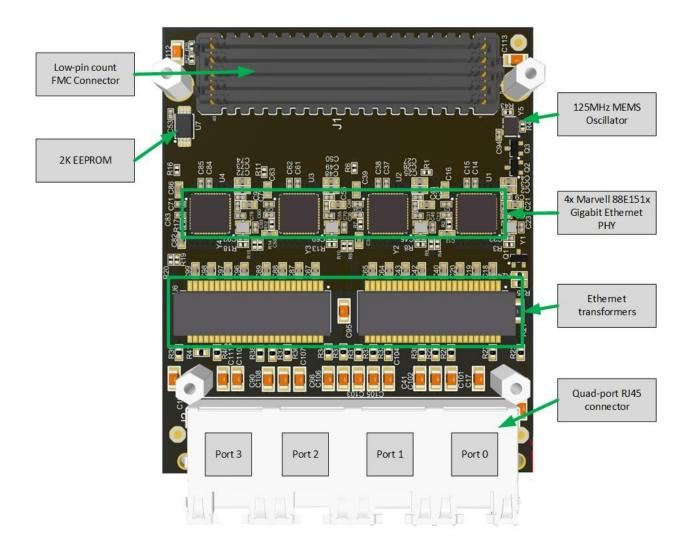
The main components on the top-side of the mezzanine card are:
