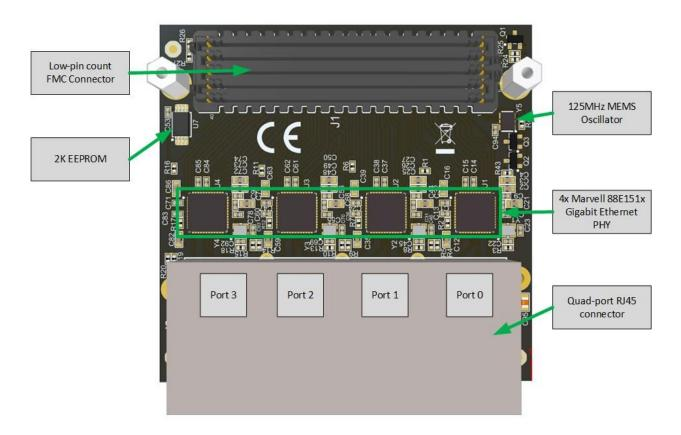
The main components on the top-side of the mezzanine card are:
