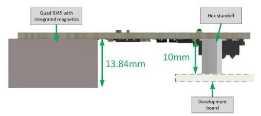
The figure below displays an example of a carrier board with an FMC connector that is located in close proximity to the board edge. The Ethernet FMC is limited to mating with this type of carrier board only.
