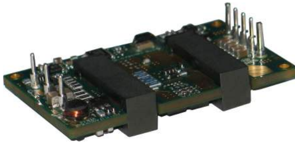
Industry standard quarter brick (open-frame) 2.28" × 1.45" × 0.39" (open-frame) 2.28" × 1.45" × 0.5" (with baseplate)
