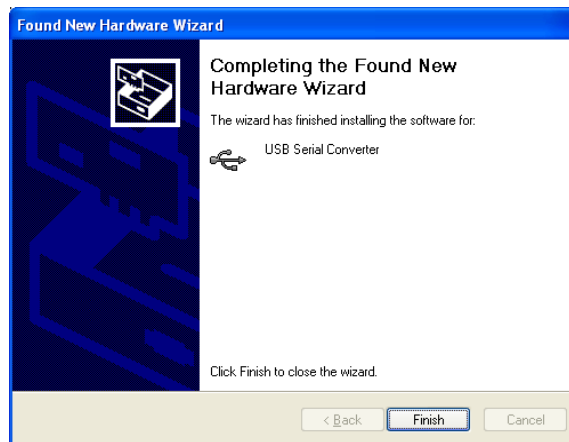
Figure 2.6 - Complete Hardware Installation
