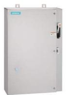
Non-reversing motor starter Size 3 Three phase full voltage Solid-state overload relay OLRelay amp range 25-100A 240VAC 50HZ / 277VAC 60HZ coil Combination type 200A fusible disconnect 200A/250V fuse clip Encl NEMA type 4X 304 S-steel Water/dust tight non-corrosive Extra-wide enclosure
