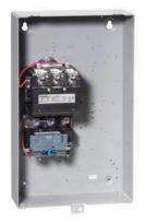
Non-reversing motor starter, Size 3 1/2, Three phase full voltage, Solid-state overload relay, OLR amp range 50-200A, 208VAC 60Hz coil, Non-combination type, Enclosure type 1, Indoor general purpose use, Standard width enclosure
