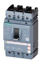
molded case switch 3VA5 UL frame 250 max. sh-circ breaking capacity 100kA @ 480 V 3-pole, line protection MCS110, In=250A without overload protection self-protection li=10 x In cable connection on both sides
