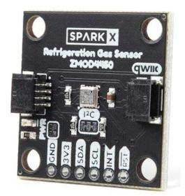
sulfide ( $C_2H_8S$ ) in air with up to ±10% repeatability and with additional calibration using a known organic compound can be accurate to ±15%. With the ZMOD4450 you can finally quantify that funky smell coming from your refrigerator.
