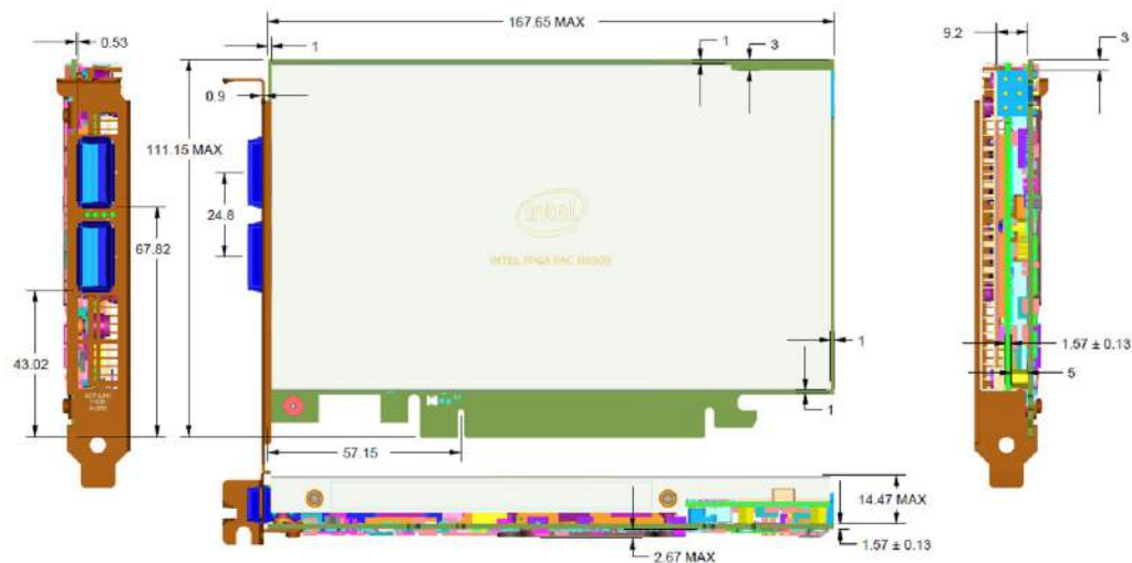
Figure 4. Intel FPGA PAC N3000 Dimensions
