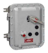
Non-reversing motor starter, Size 1 3/4, Three phase full voltage, Solid-state overload relay, OLRelay amp range 10-40a, 110V 50HZ / 120V 60HZ coil, Combination type, 60Amp non-fused disconnect Encl. NEMA type 4X Fiberglass Water/dust tight noncorrosive, Standard width enclosure
