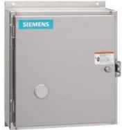
Non-reversing contactor, Size 2 1/2, Three phase full voltage, Contactor amp rating 60A, 3 wire (NO aux included), 220-240/440-480VAC 60Hz coil, Non-combination type, Encl NEMA type 4X 304 S-Steel, Water/dust tight noncorrosive, Extra-wide enclosure
