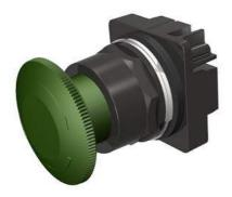
30mm BlackMax, Epoxy Coated Corrosion Resistant Metal Operator, Round Twist-to-Release Operator Non-Illuminated Mushroom Head Cap Small 1.79" (45 mm) Plastic Cap, Green 2 Position Maintained, Twist-to-Release UL Listed, CSA Certified NEMA 1,3,3R,4,4X,12,13 & Automotive Standards
