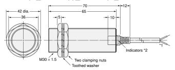
\*1. 6-dia. vinyl-insulated round cable with 2 conductors (Conductor cross section: 0.5 mm<sup>2</sup>, Insulator diameter: 1.9 mm), Standard length: 2 m 6-dia. vinyl-insulated round cable with 3 conductors
