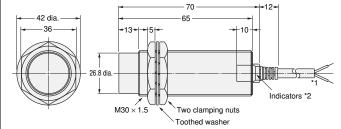
\*1. 6-dia. vinyl-insulated round cable with 2 conductors (Conductor cross section: 0.5 mm<sup>2</sup>, Insulator diameter: 1.9 mm), Standard length: 2 m 6-dia. vinyl-insulated round cable with 3 conductors
