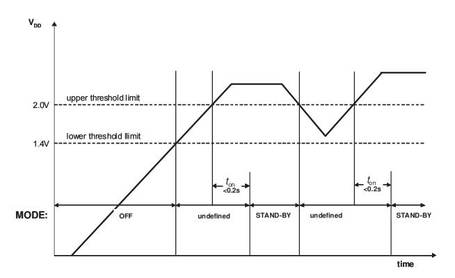
The threshold limit where the device switches from OFF to STAND-BY mode is between  $V_{\text{DD}}$  =1.4V and  $V_{\text{DD}}$  =2.0V.
