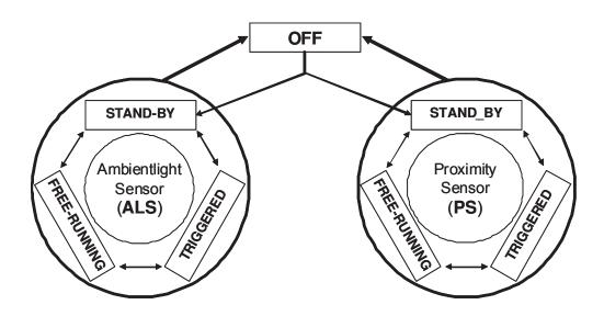
If  $V_{\rm DD}$  exceeds the threshold-voltage, the sensor will switch from OFF mode to STAND-BY mode. As shown in the transition-diagram above it is possible to switch between all modes without any restriction. The transition time between modes ( $t_{\rm trans}$ ) is < 10ms. The delay time between STAND-BY and start of measurement is max. 10ms for the ambient light sensor.
