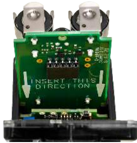
Figure 1. Q45 battery board
