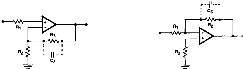
FIGURE 4. SUGGESTED STABILITY CIRCUITS
