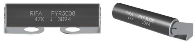
The PYR resistors are wire wound on a ceramic core and coated with high temperature silicone. The mounting brackets are made of stainless steel and connected by two point spot welding.
