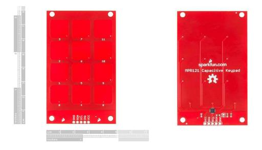
**Description:** The MPR121 capacitive keypad uses the MPR121 and 12 touch sensitive pads to give you a simple 'keypad' with an I<sup>2</sup>C output. These keypads function by measuring the capacitance of twelve electrode points. When an object comes close to the electrode connector, the measured capacitance changes. This signals the MPR121 that something has touched a 'button'.
