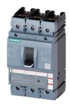
circuit breaker 3VA5 UL frame 250 breaking capacity class C 100kA @ 480 V 3-pole, line protection TM230, FTAM, In=175A overload protection Ir=175A fixed short-circuit protection Ii=5...10 x In cable connection on both sides
