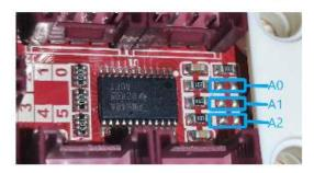
After soldering a 0 ohm resistor, the corresponding pin will change from low to high, and the pin level combination and its corresponding I2C address are shown in the table below.
