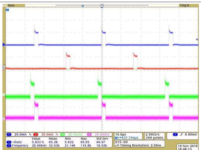
Figure 80. Current Waveform of OUT0, OUT1, OUT2 and OUT3
