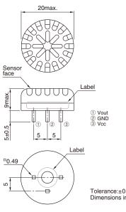
Tolerance:±0.2mm Dimensions in mm
