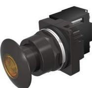
30mm BlackMax, Epoxy Coated Corrosion Resistant Complete Metal Unit Illuminated Push-Pull Operator Transformer type, 600V AC Incandescent Lamp Mushroom Head Cap Small 1 3/4" (44.5 mm) Metal, Black with Amber Lens 3 Position Pull-Momentary/Push-Maintained UL Listed, CSA Certified NEMA 1,3,3R,4,4X,12,13 & Automotive Standards
