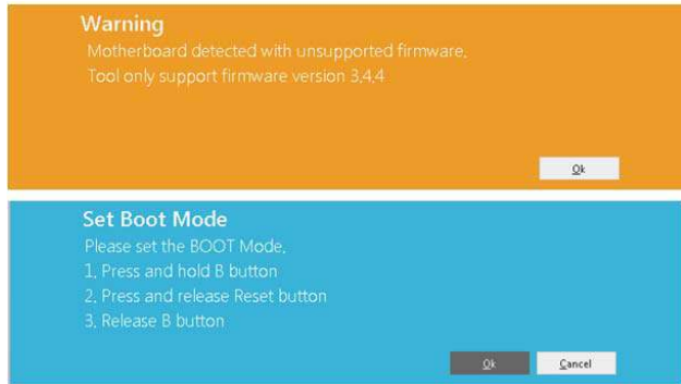
Figure 7. Updating the EVAL-ADPDM3Z Evaluation Board Firmware
