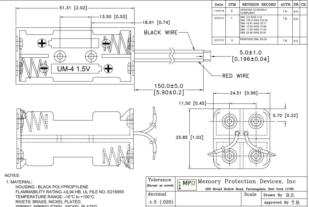
SPRING: SPRING STEEL, NICKEL PLATED. CONTACTS: SPRING STEEL, NICKEL PLATED. WIRE: 26 AWG, UL1007, CSA, TR64, 300V, 80°C CONTACT RESISTANCE: UNDER 50mΩ FOR +/- CONTACTS PER EIA-540J000
