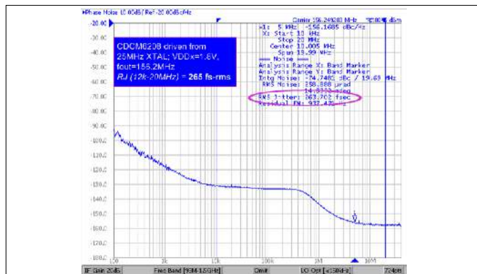
Figure 2. Typical Device Output Phase Noise and Jitter for 25 MHz
